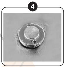
Make the NMO Mount flat in the vehicle surface.
