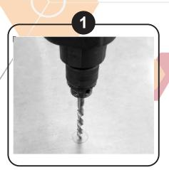
Using a 3/4" hole saw, make a hole in the vehicle roof where the center of the antenna will be installed.
