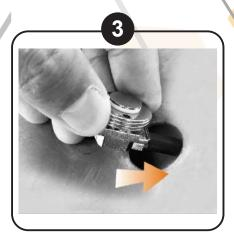
Insert the rear side of the NMO mount inside the 3/4 inch hole.
