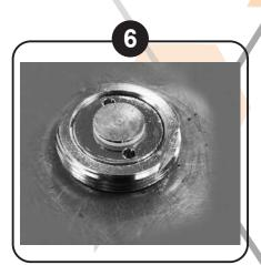
Done and make sure the gasket is seated to the vehicle surface
